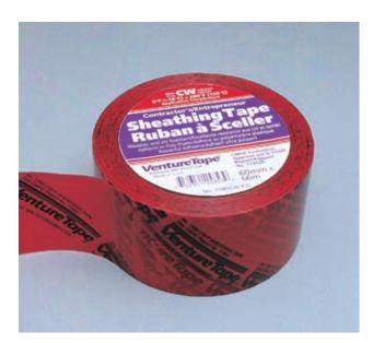
Venture Tape<sup>®</sup> 1585CW<sup>®</sup>-P2 is a printed polypropylene sheathing tape coated with an aggressive acrylic pressure sensitive adhesive (PSA) designed for use as a closure system and vapor seal on all interior and exterior sheathing materials.
