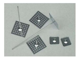
TACTOO® Insul-Hangers have 12 ga (.106"/2.7mm) diameter mild steel spindles with a corrosion resistant coating. The perforated base plate is 2" (51mm) square and is made of galvanized steel. Standard lengths range from 1" (25mm) through 9 1/2" (241mm) and are packed 1,000 pieces per carton up to 2 1/2" (64mm); 500 pieces per carton for longer sizes.
