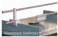
Installation is easy: The S-5!® clamp mechanically attaches to the panel seam by inserting and tightening our patented round-point setscrews to the specified tension (see www.S-5.com). These screws will slightly dimple the seam material, but not pierce it. Our patented clamps offer durability unequaled by chemical bonds and adhesives that degrade with time and exposure.
